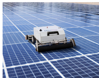
Figure 6 — The automated cleaning robot eliminates localized soiling and helps control vegetation growth
